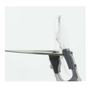
Hold lens fixation firmly with mounting pliers
