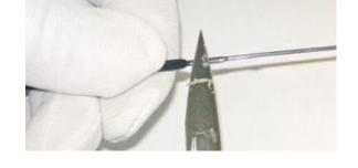
5. Cut temple tip to desired length with sharp blade, using trimmed metal piece as sizing guide
